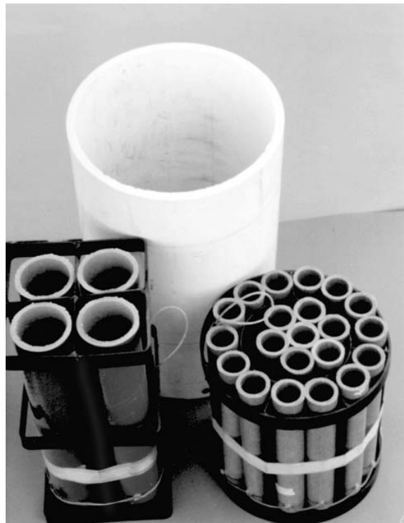
Photo 4. View of small one and two inch mortar frames and heavy walled plastic tube used to protect adjacent mortar when firing small salutes.
