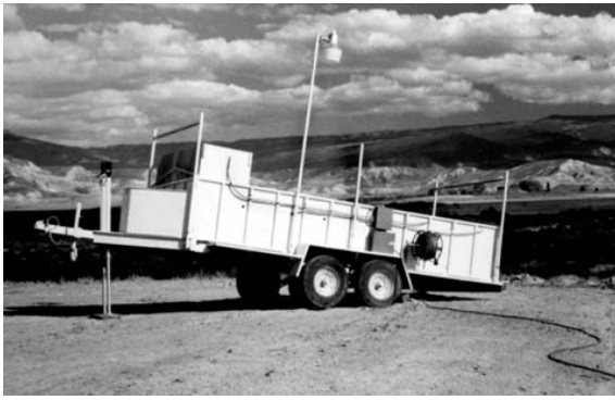
Photo 1. Side view of large "Dense-Pack" mortar trailer raised into possible firing position.
