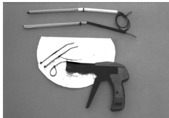
Photo 5. "Chain Fusing" components. Shown are: match headers attached to a piece of shell leader; delay fuse link attached to a piece of shell leader; aluminum foil / fiberglass mortar cap, folded to show both its sides; small cable ties and a tensioning tool.
